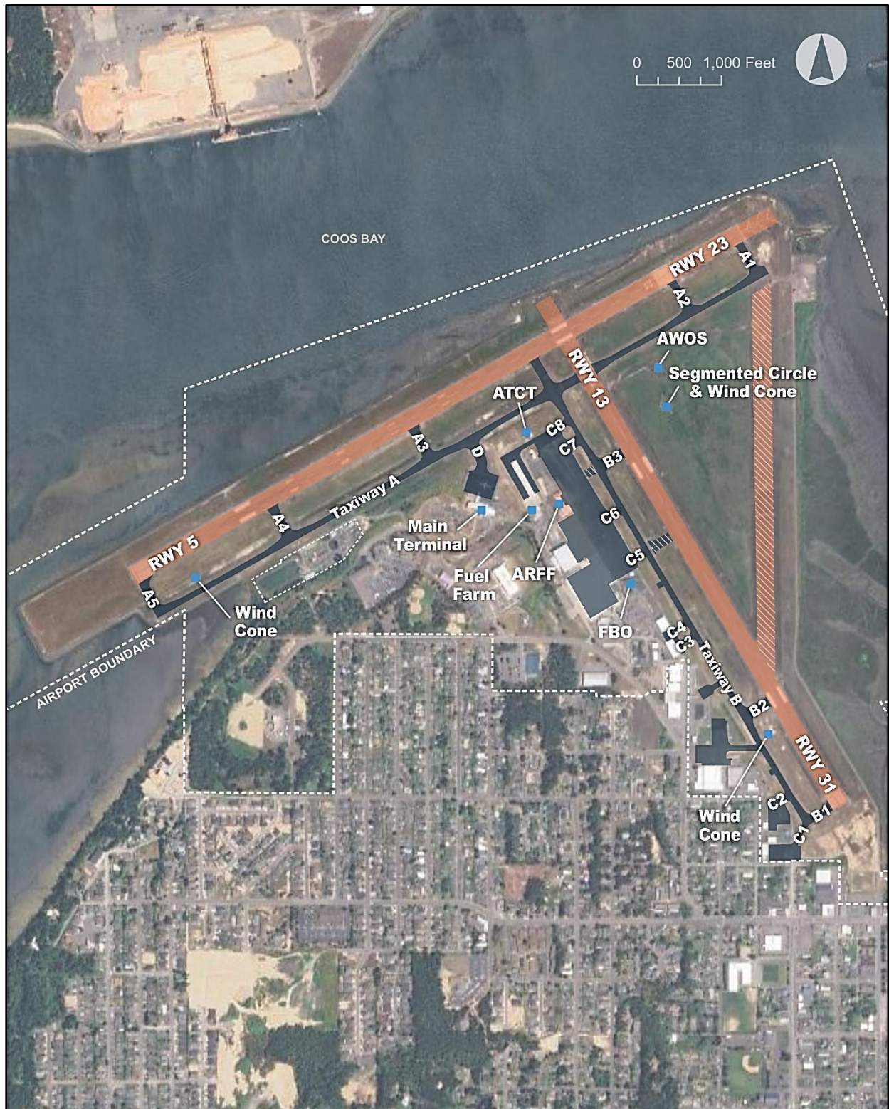
Figure 1-3 Airport Facilities Southwest Oregon Regional Airport
